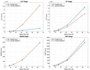
To enable a more valid comparison, the vector multiplier was modified to include pipelining. For smaller matrices (N=8, N=16), a single-stage pipeline was introduced just before the adder tree. For larger matrices (N=32), an additional pipeline stage was added at the level 2 adder of the adder tree, resulting in a two-stage pipeline. This modification allowed the design to meet the 100 MHz timing constraint successfully.
