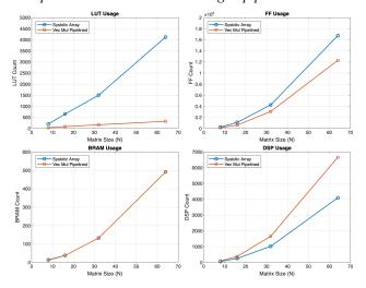
To reduce excessive LUT usage in pipelined paths, the use\_dsp flag was applied. The higher LUT utilization in systolic arrays compared to vector multipliers is mainly due to the data setup controller, not the computation units.
