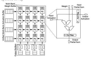
A systolic array is a control-minimized methodology based on processing elements (PEs). Each PE contains a MAC (Multiply-Accumulate) unit and performs computations as long as data flows are provided in sync with the timing requirements. The key advantage of systolic arrays lies in their minimal data control overhead.
