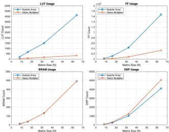
For a non-pipelined vector multiplier, the FPGA resource utilization is significantly lower compared to a systolic array. This difference arises because the systolic array inherently incorporates pipelining within its architecture and requires additional logic to set up input data and align output data for results, leading to higher resource consumption.
